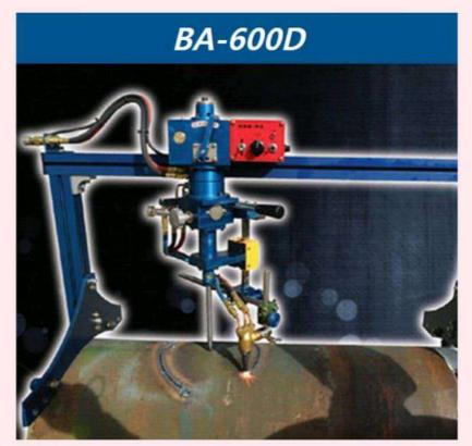
The machine torch mounted on KHC-600D can cut circular shapes vertically when mounted on flat surface and cut bevel Circle when mounted on curved surface of storage tank or heat exchanger through its unique lever mechanism saving substantial labour in marking, manual cutting & surface grinding
